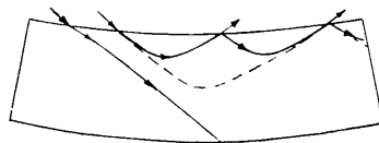
Fig. 4. Ray trajectories in a bent crystal. The Bragg diffraction case.
